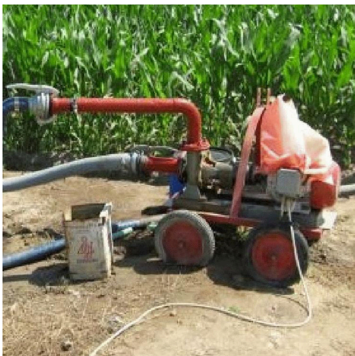
Electric water pump that provides irrigation water directly from canal (Alexandros Pechtelidis)
