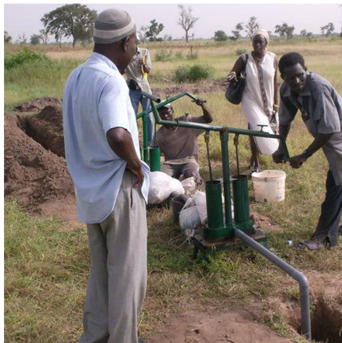
Hand pump for supply of irrigation water (Sourakata Bangoura (Land and Water Resources Officer for Central Africa, Libreville, Gabon))
