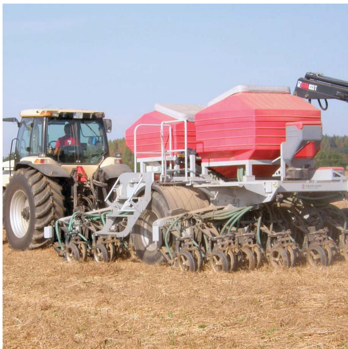
Sowing into the last year plant residues with CROSS-SLOT seeder (Peeter Viil)
