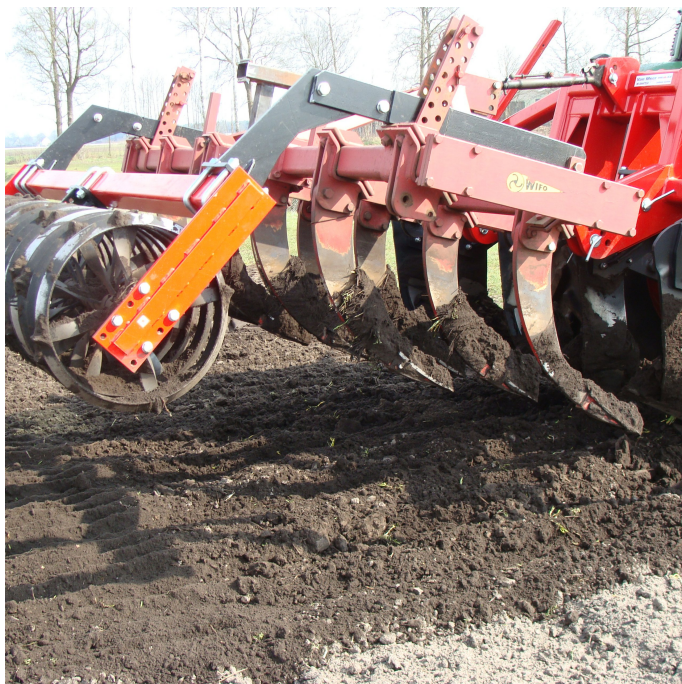
Close up of the non-inversion tillage machine. The pens in the front penetrate and thereby loosen the soil, the wheel at the back rolls over the soil to compact it a little bit at the end. (Harry Verstegen)
