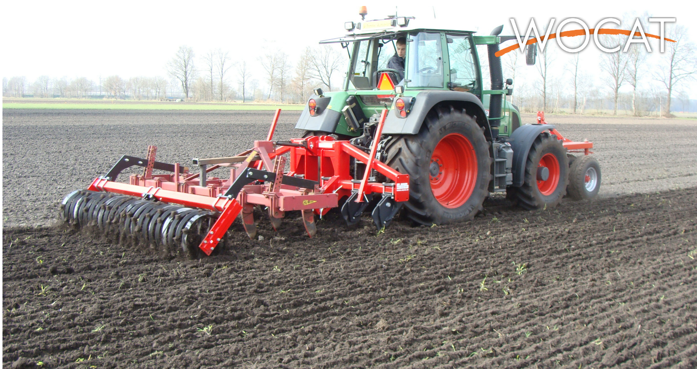
In the picture you see the machine that is used for non-inversion tillage (Harry Verstegen)
