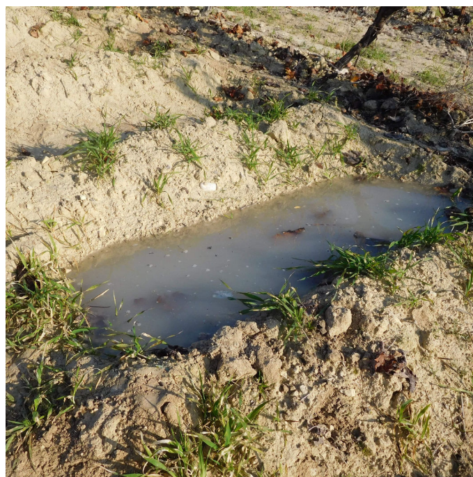
Some aserpias were filled with water for infiltration tests. (Gema Guzmán)
