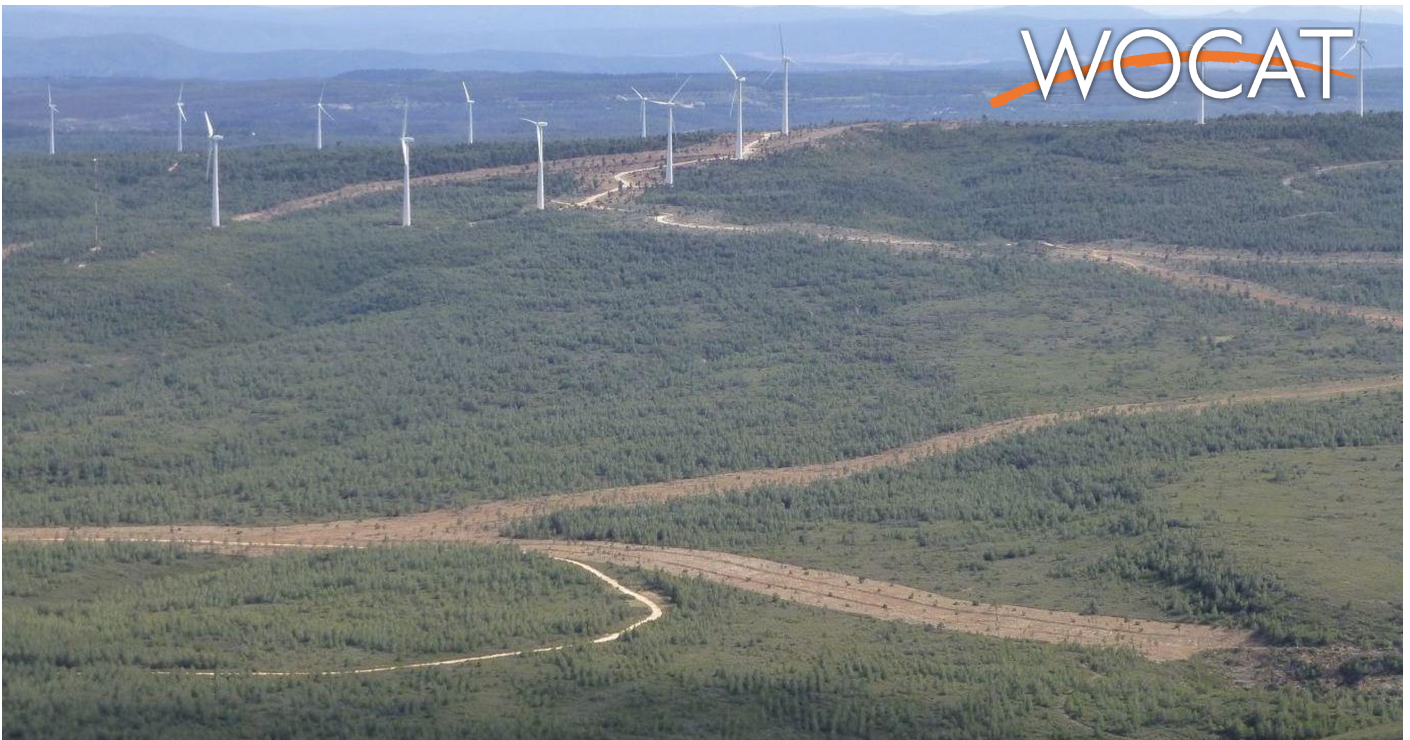
Firebreaks are classified in first, second and third order, together forming a system isolating separate areas by wide strips. This parcelling aims in controlling the spread of large forest fires. (Nina Lauterburg)
