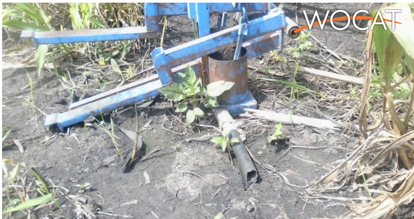
A treadle pump used for low-cost irrigation. (Charles-Lwanga Malingu)
