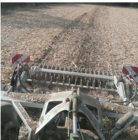
Tillage with a disk harrow after mulching maize residues left on surface. Preparation for sowing with a combined seeder. (Andrej Ropić)
