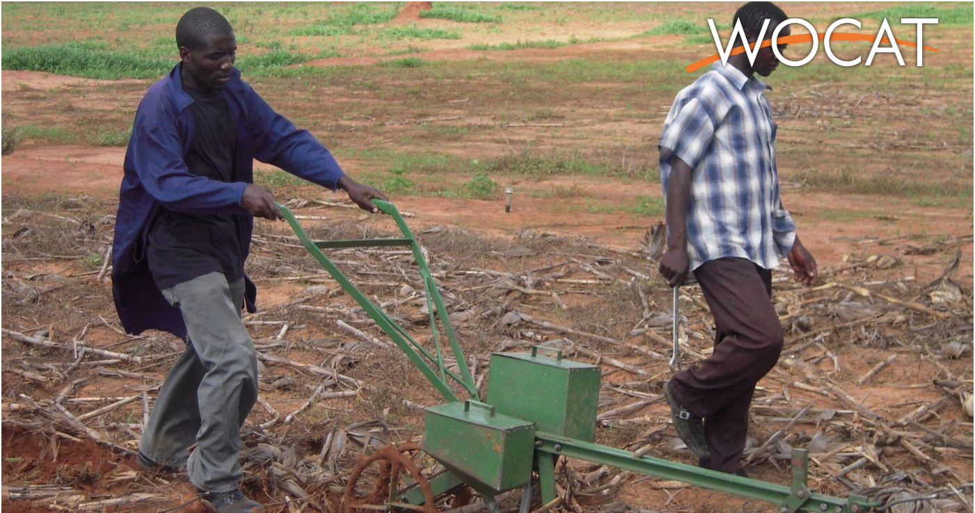
The Magoye CA planter used for Zero-tillage (Arthur Chomba (Box 670577, Mazabuka, Zambia))
