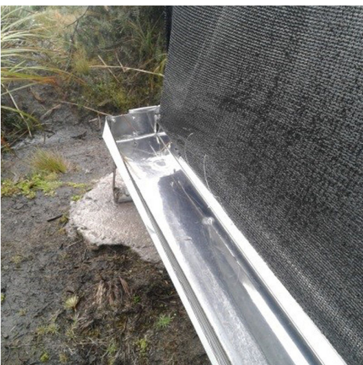
Fog Water Capture System (Carol Tapia)
