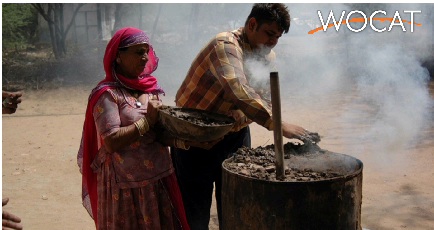
Household production of biochar using diverse feedstock (World Agroforestry)
