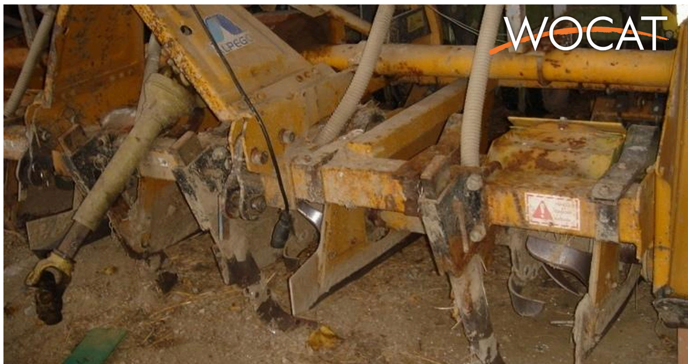
Maize strip tillage machine with gruber (A) und Fräse (B) (Giulietta Buddeke)
