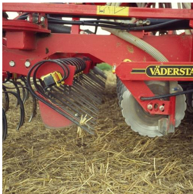
Detailed view of the 'Väderstad Rapid Cultivation Drill' with tines and discs. (Alastair Leake)
