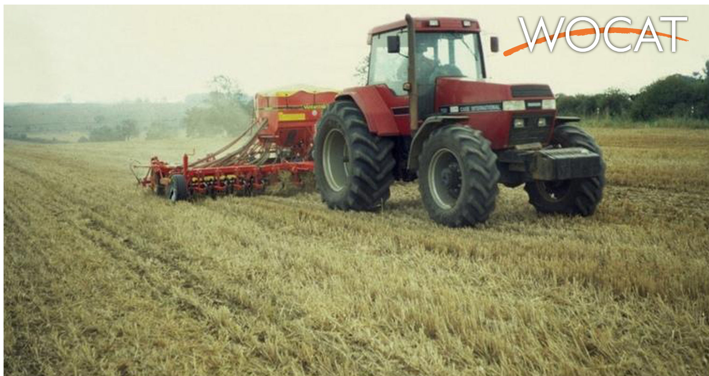
A tractor with the 'Väderstad Rapid Cultivation Drill' in action: a light surface tillage followed by direct seeding. (Soil and Water Protection, SOW)
