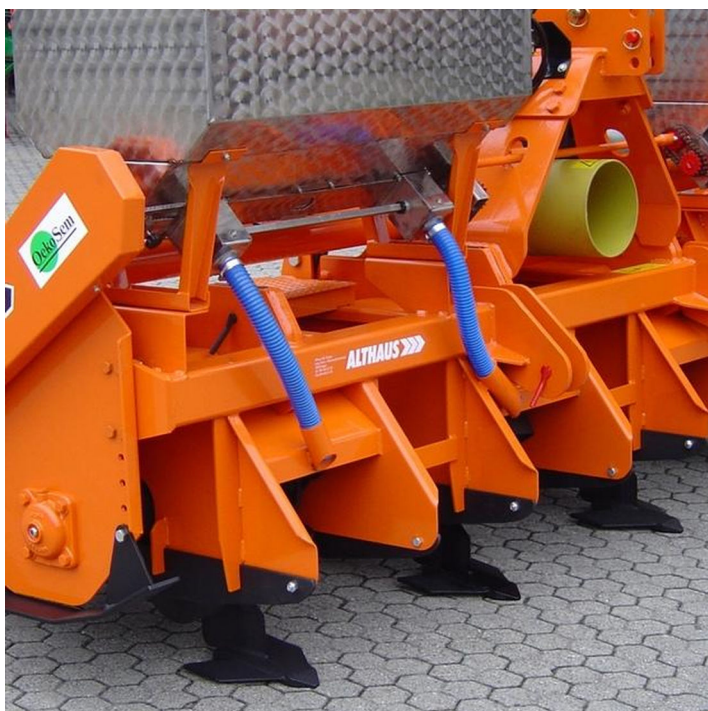
The machine includes a rotary tiller, manure distributor and grubber. The spraying device is not shown. (Althaus AG (Ersigen, Switzerland))
