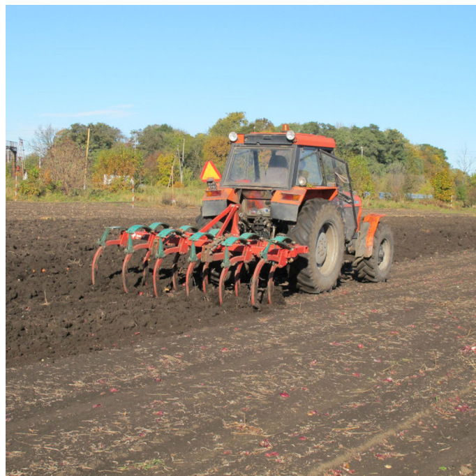
Tractor with subsoiler in action (Zygmunt Miatkowski)
