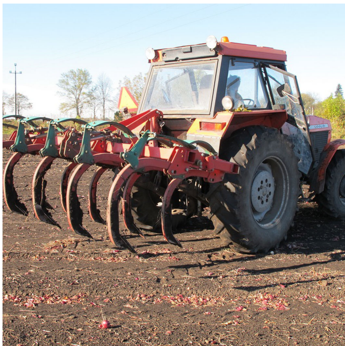
Tractor with subsoiler in action (Zygmunt Miatkowski)
