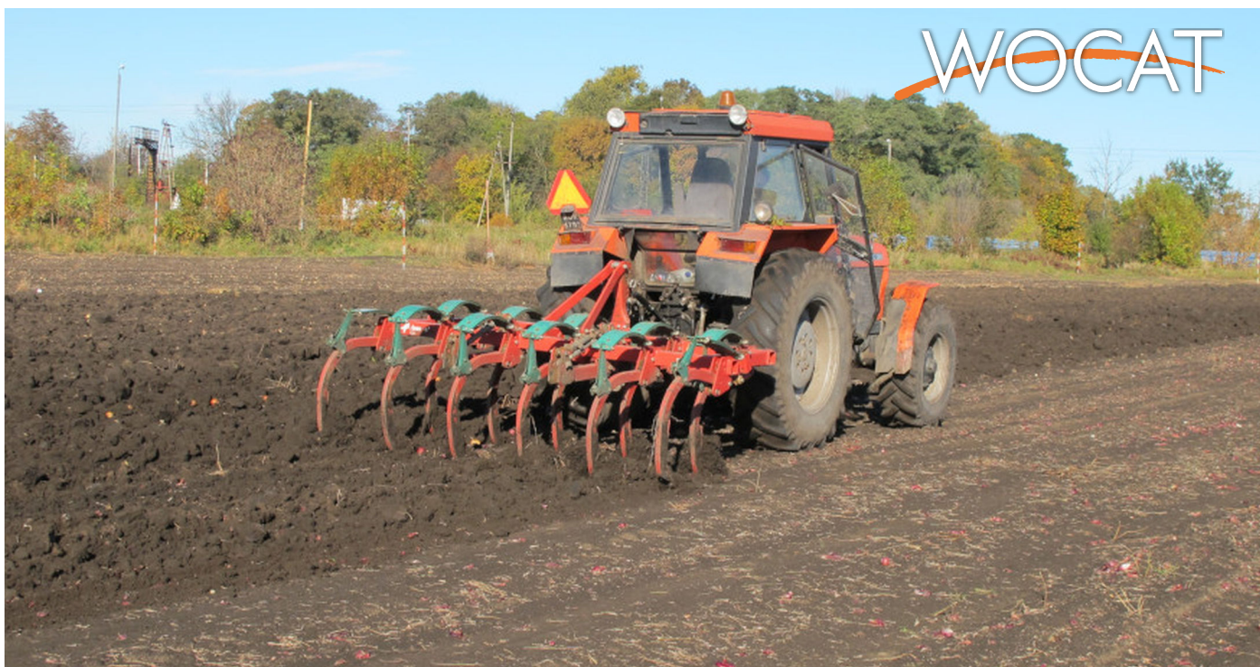
Tractor with subsoiler performing tillage (Tymoteusz Bolewski)
