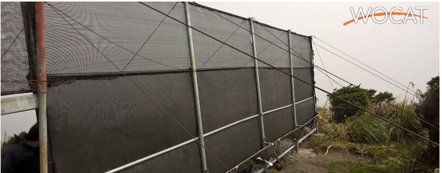
Fog water capture system (Carol Tapia)
