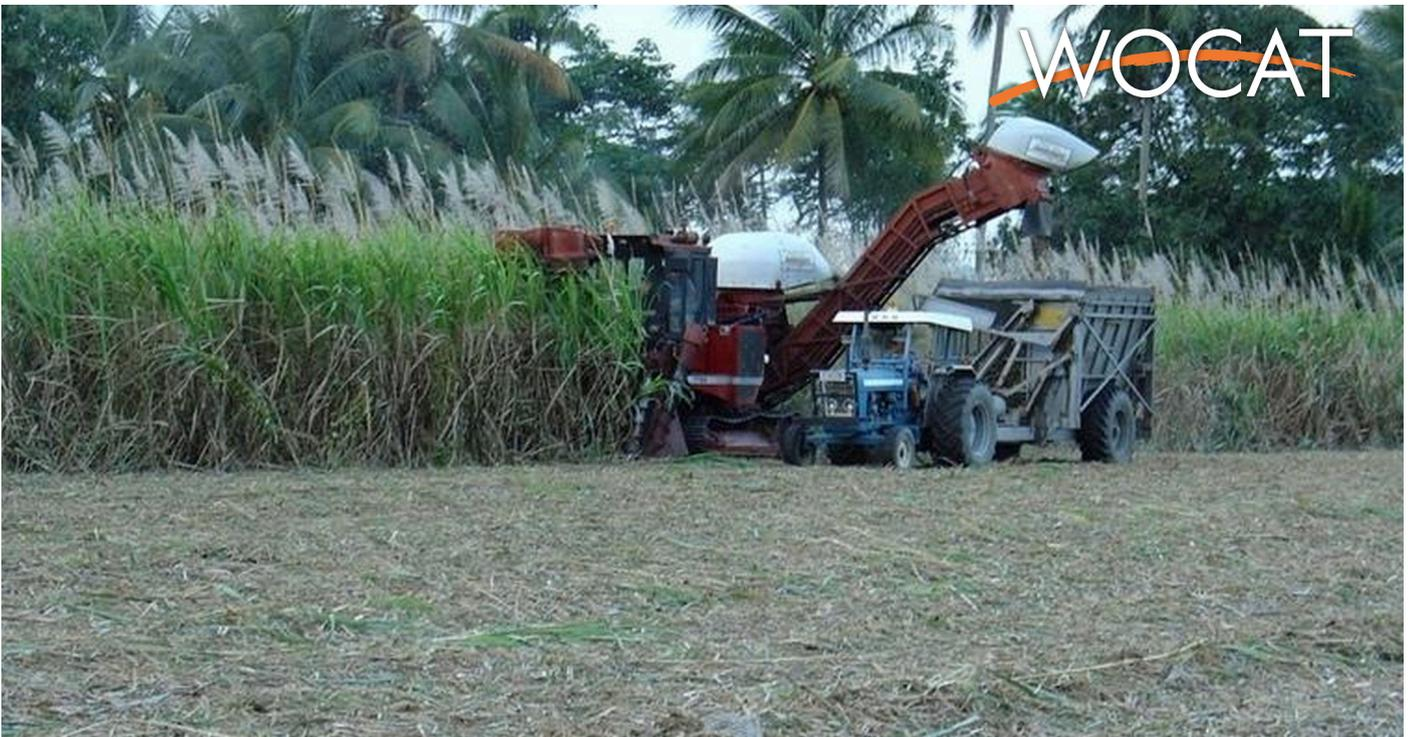
Harvesting of green sugar cane and simultaneous spreading of the separated residues, leaving a dense mulch cover, the so called green cane trash blanket. (Hanspeter Liniger)
