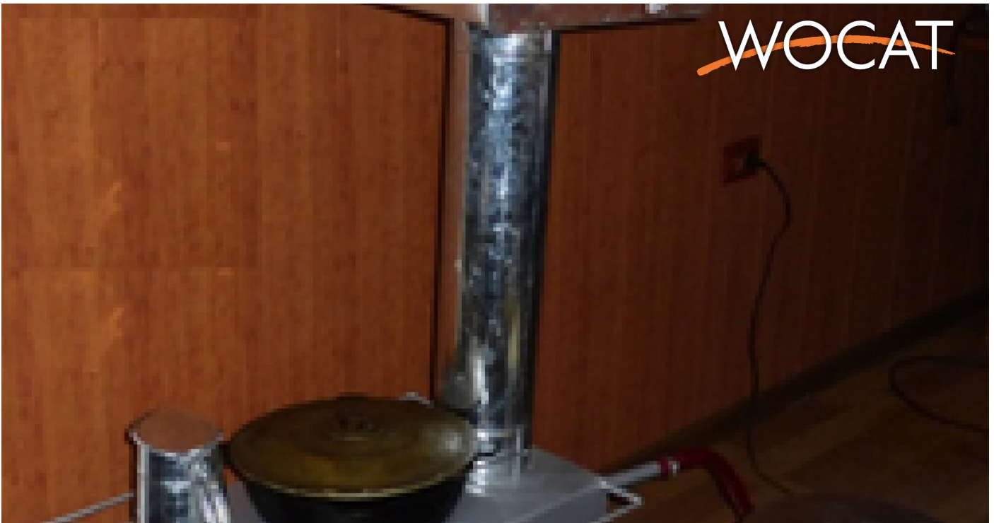
Modified stove assembled with heat-exchanger and water tank (Daler Domullodzhanov)
