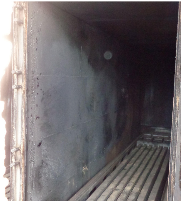
Burning and heating chamber for wood pyrolysis (Beatrice Adoyo)
