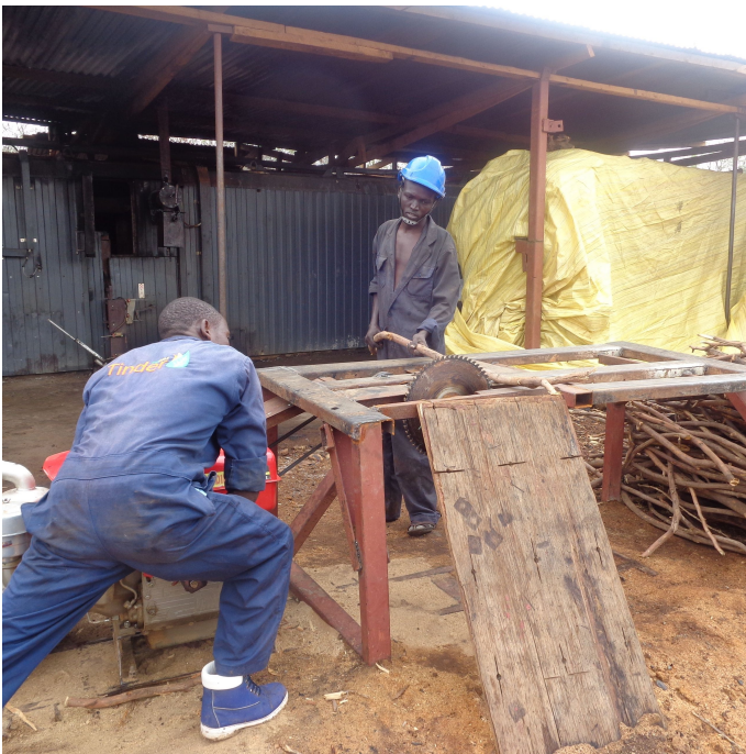
Prosopis wood being cut into 15 cm lengths for loading into trolleys (Beatrice Adoyo)
