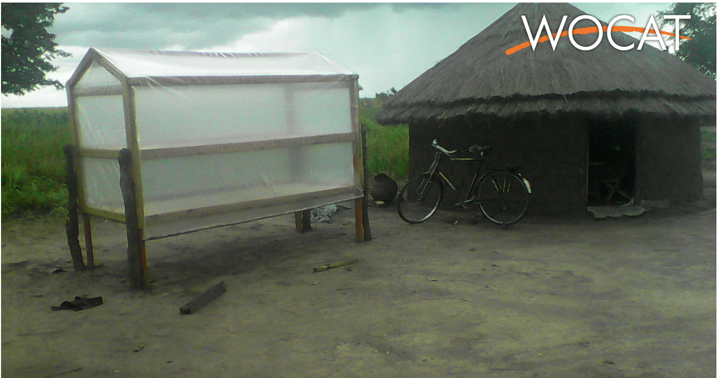
Wooden frame solar dryer placed in the farmer's compound (Amale Balla Sunday)
